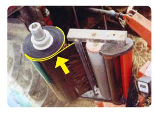
The film roll has over-run here, allowing the film to touch and stick together, as shown by the high-lighted edge of the film in the picture.
