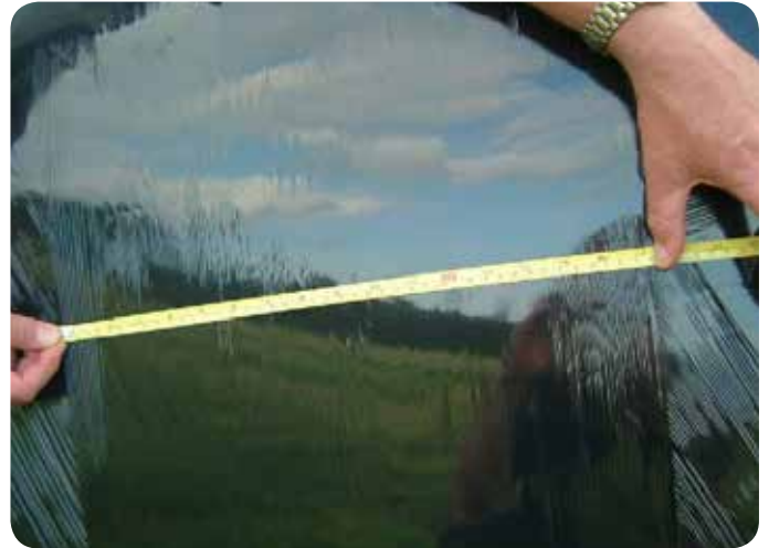
The film 'neck-down' can be checked by measuring the film width across the end of the bale.
