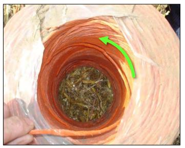
The spool MUST be used the correct way up, so that the twine pulls from the spool in a Counter-Clockwise direction.
