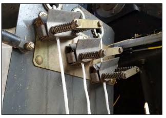
Adjust the twine tensioners at the twine box with slight tension to prevent twine free falling. Ensure twine tension plates are kept clean and free from crop debris, which if allowed to build up between the plates, can reduce the twine tension
