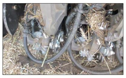
Ensure knotters are free from dust and crop residue, which can interfere with knotting process
