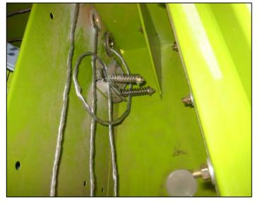
If the twine is pulled from the wrong end of the spool, it will increase the twist, creating loops that can become trapped on the internal parts of the baler.
