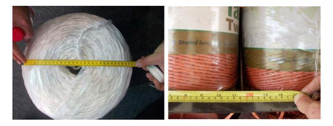
Ensure the spool is not too tall, and can fit easily below the twine guides in the top of the twine box on the baler. If there is insufficient space above the spool, the twine may not be able to pull freely from the spool.
