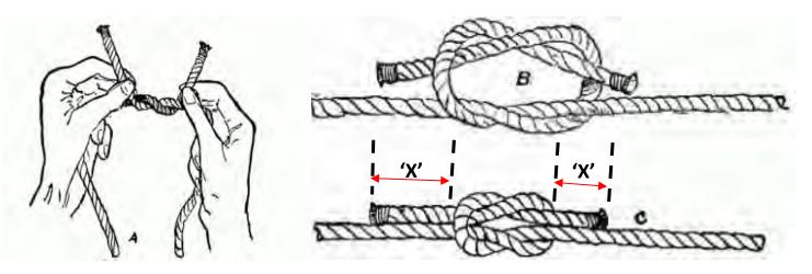
Tails on spool joining knot ('X') should be 15 – 20mm after tightening
