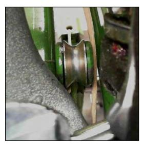
Ensure the needle wheels are free turning and are correctly aligned with the bill-hook and that twine is not outside the needle wheels
