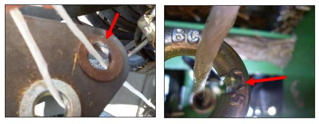
Worn or damaged guides can damage the twine, breaking fibres and reducing the twine strength.
