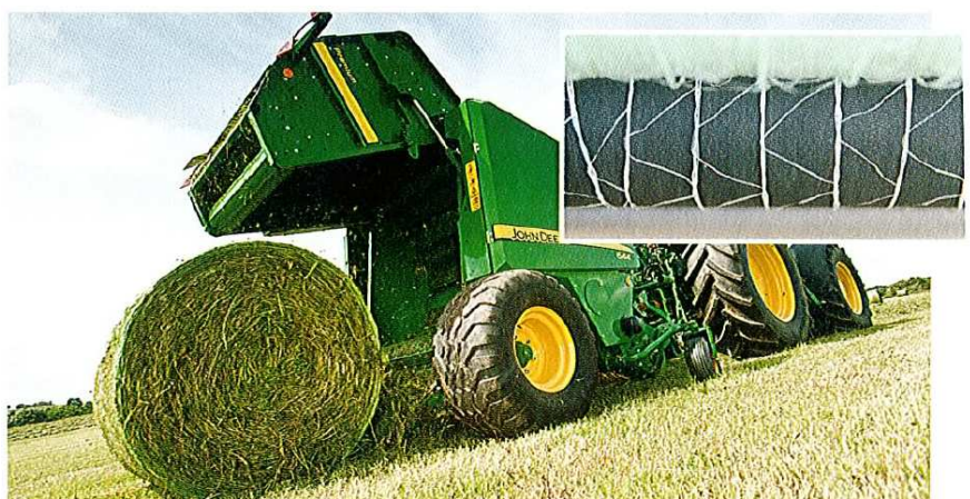
The Schuss-threads of the Tama nets are waved and therefore elastic. Because of this the net does not run in when running on the bale and also the shoulders are covered.
